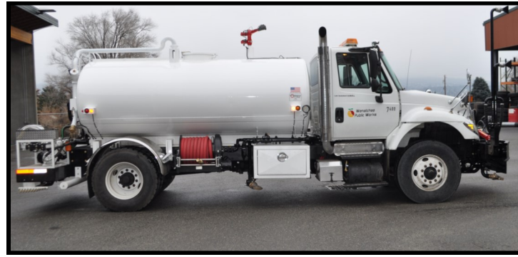
Hydrostatic drive 2,200 gallon stainless steel flusher with sidewalk flusher, OMCO deicer with raven controls, monitor, gravity bar, rear spray heads, hose reel and quick change suction hose
