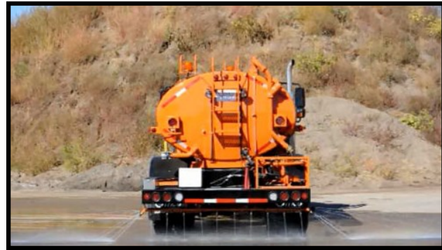
Hydrostatic powered OMCO 2,500 gallon stainless steel tank flusher / deicer with Robo Flush™. OMCO deicer system with Force America control system
