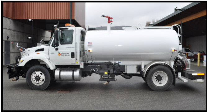
Hydrostatic drive 2,200 gallon stainless steel flusher with sidewalk flusher, OMCO deicer with raven controls, monitor, gravity bar, rear spray heads, hose reel and quick change suction hose
