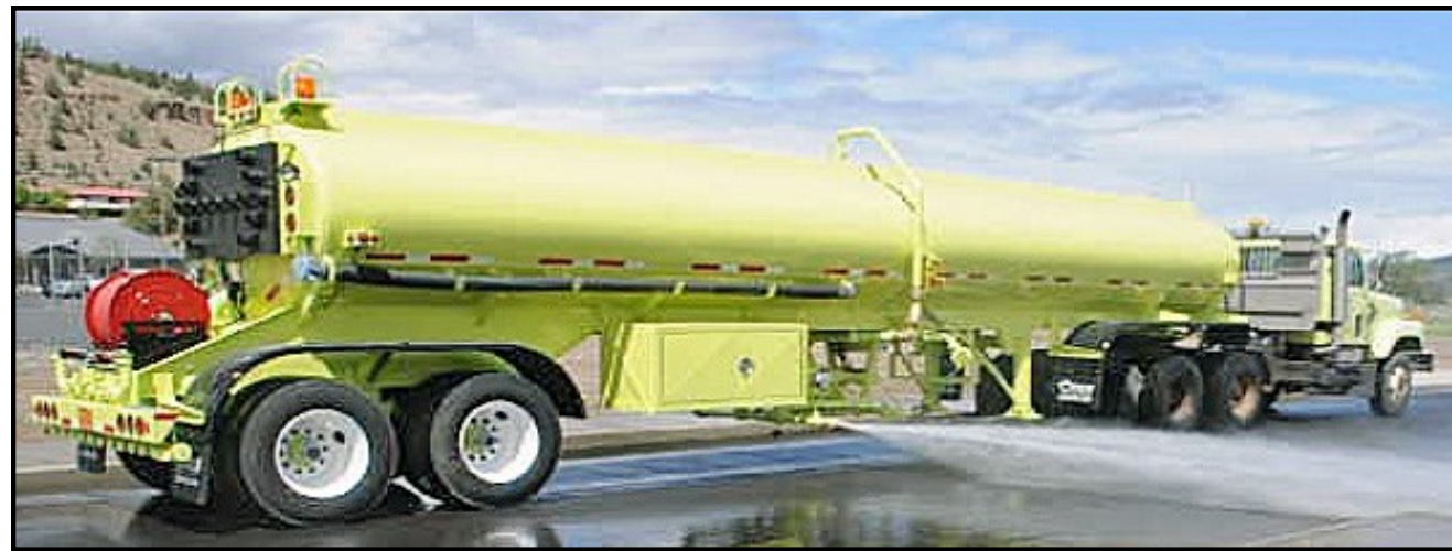
Hydrostatic powered OMCO 6,000 gallon stainless steel tank , 40' semi trailer. Self priming water pump, flusher, deluge, spray heads, hose reel, gravity bar, fire discharge and deicer capabilities. Just to name a few.
