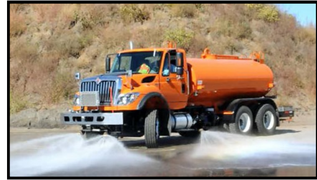
Hydrostatic powered OMCO 2,500 gallon stainless steel tank flusher / deicer with Robo Flush™. OMCO deicer system with Force America control system
