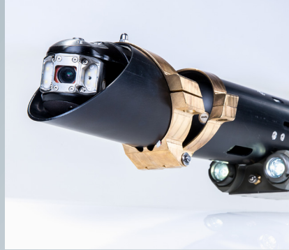
Top: LATRAS guiding system for positioning camera for launch. Left: LATRAS sensor with jetting nozzle Above: Automated visualization of LATRAS data in software
