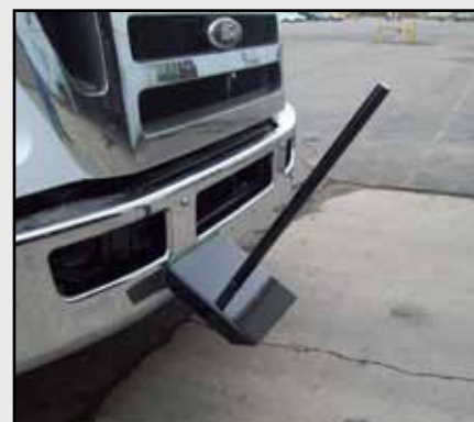
Bumper mounted Cone Holders save space and increase visibility.
