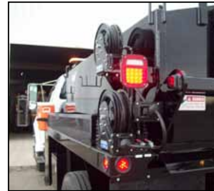
Air and solvent wands aid in clearing debris from potholes prior to sealing and patching.
