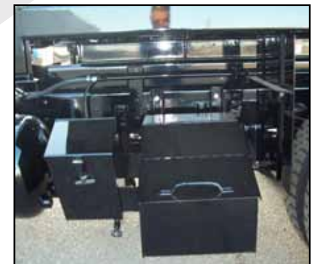
Sand box carries base material for deeper potholes and a solvent dip tank to clean tools before and after patching.
