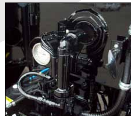
Electric and propane heater systems are available to keep emulsion systems hot around the clock.
