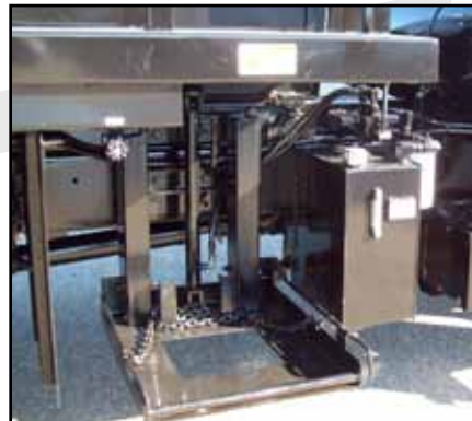
Optional vibratory plate hydraulic platform to reduce back injuries relating to lifting hazards.
