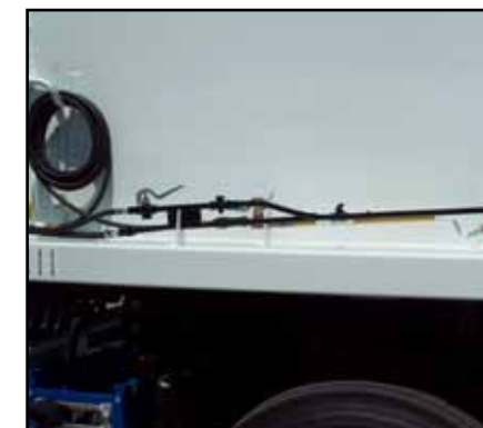
Emulsion wand stores securely in combination with waste tank to separate waste from usable material.
