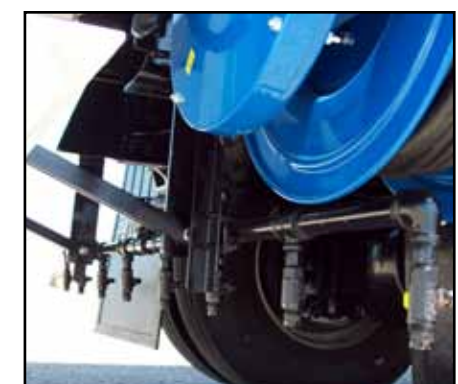
Spray bars allow your pothole patcher to double as a liquid asphalt distributor when necessary.
