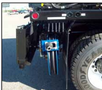
Rear ergonomic controls and pneumatic lines located curb side to keep workers away from traffic hazards.
