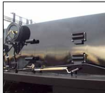
200,000 BTU hand torch eliminates moisture from potholes prior to sealing and patching.
