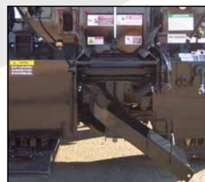
Pivoting Asphalt Chute
