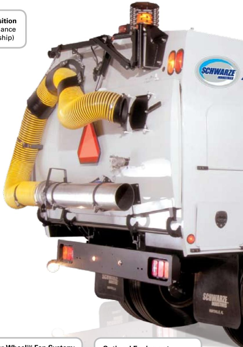
The Schwarze A7 Zephyr is a chassis mounted, regenerative air runway sweeper with an 8.4 cubic yard hopper. With over 20 years of successful operation throughout the world, the A7 Zephyr is a heavy duty workhorse that will provide a high quality option with a low cost of ownership. Come to the people you know, for the products you trust.
