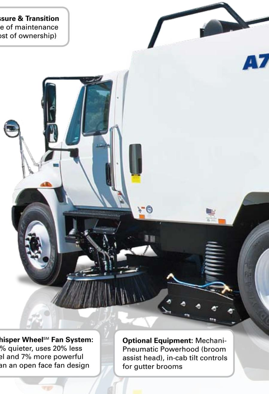
The Schwarze A7 Tornado is a chassis mounted, regenerative air street sweeper with an 8.4 cubic yard hopper. With over 20 years of successful operation throughout the world, the A7 Tornado is a heavy duty workhorse that will provide a high quality option with a low cost of ownership. Come to the people you know for the products you trust.
